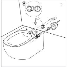
2. Insert the fixing screws as shown in the picture (Fixing pin oriented toward the installation holes of seat cover)
