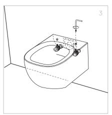
3. Tighten the pin inserting the key in the installation holes of seat cover
